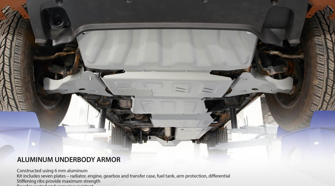
Constructed using 6 mm aluminum
